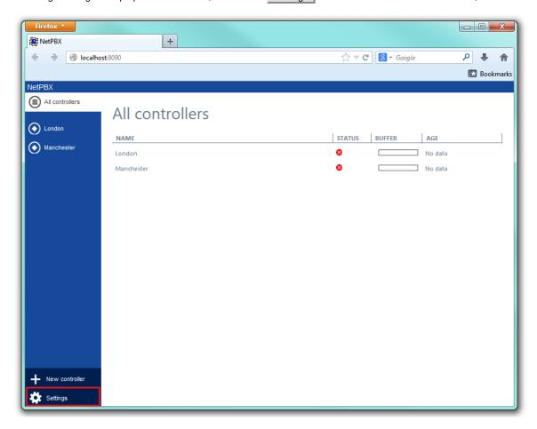
The NetPBX settings window will open, where you can configure its properties, such as IP address, port number or login credentials, as shown below:
